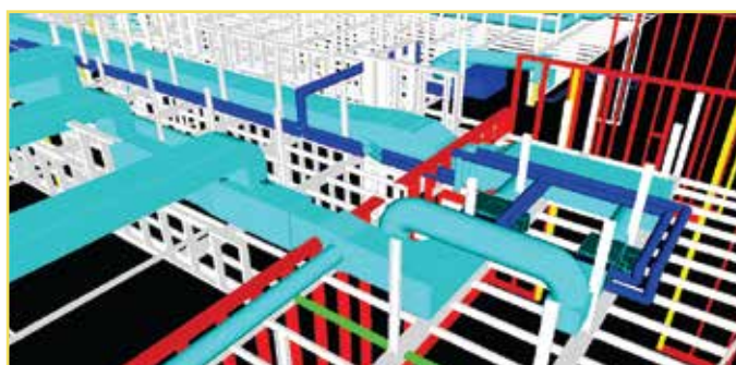
▲ Coordinated Model of Stud Framing & Mechanical
