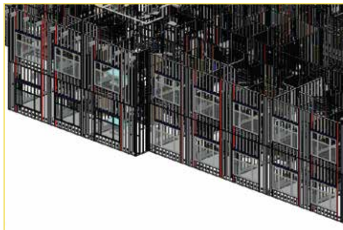
▲ Colour Coding for Critical Stud Elements
