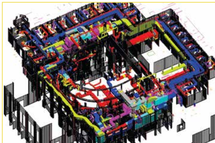
▲ Wall Framing coordinated with Mechanical trade
