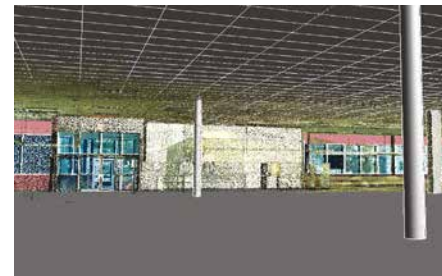
Interior view of grocery store with point cloud attachment
