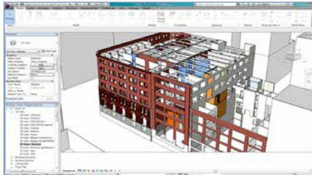
Architectural model of entire building, imported as point cloud
