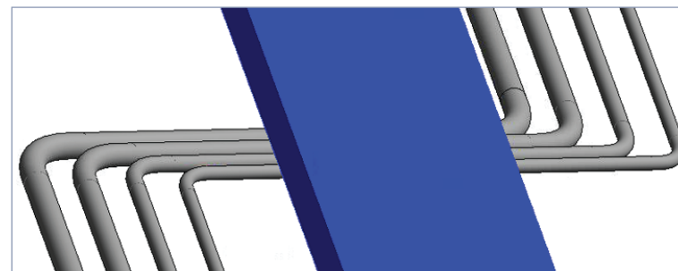
Coordination - Avoiding clash by using a rolling offset
