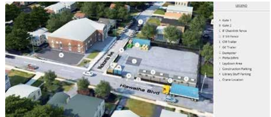
Construction Site Logistics Sample
