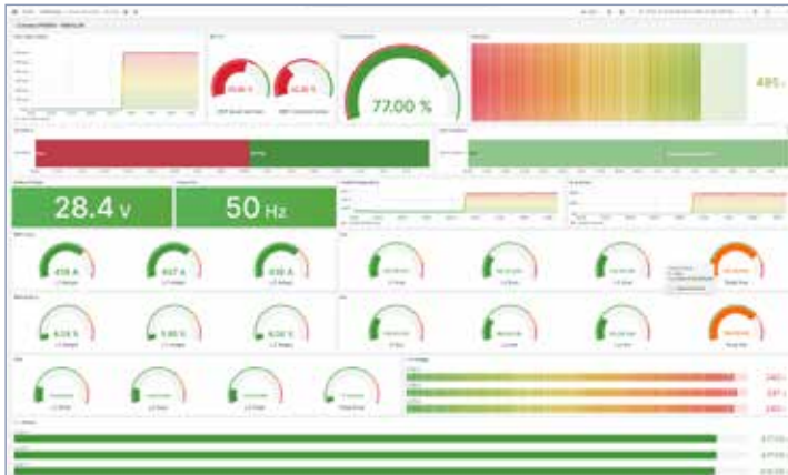
Real-time Diesel Generator Performance Dashboard (Img 2.5.1)
