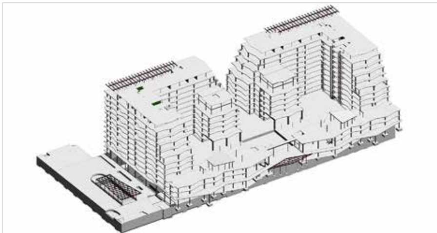
Structural BIM Model
